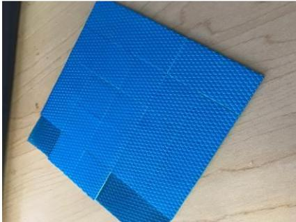
3. Peel the gap filler from the corner to make it separate from the bottom liner. Place the gap filler onto desired substrate.
