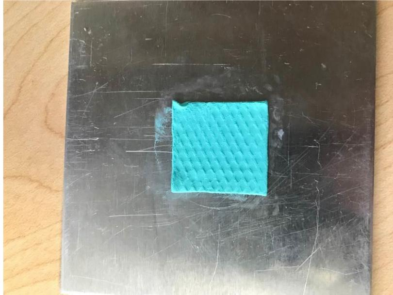
5. Cover the exposed gap filler with the diamond liner or continue the assembly process to avoid contamination of the surface from dust and debris.
