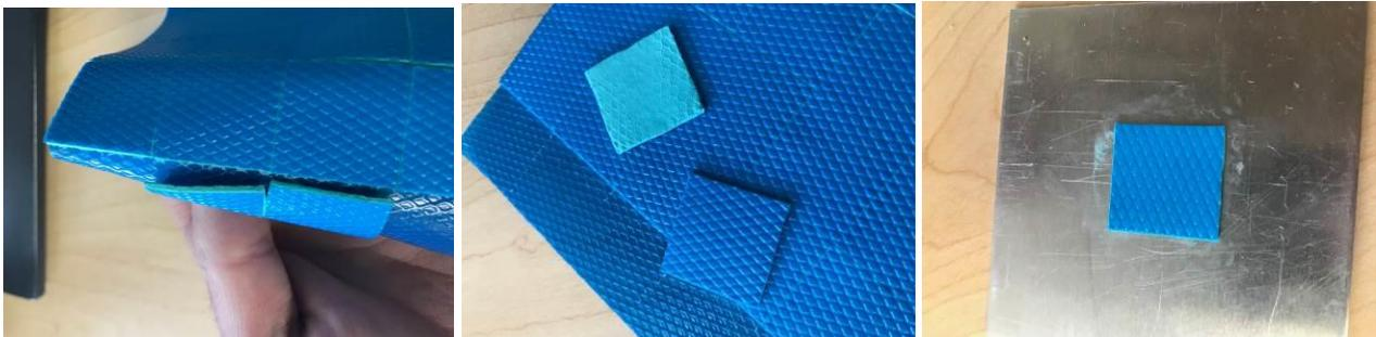
4. If liner is still on part, gently press part to adhere to substrate, then pick liner from edge and peel off in a consistent motion, leaving the part on the substrate.
