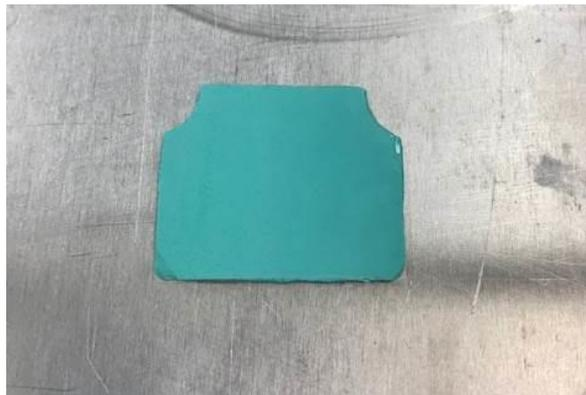
3. Peel off the remaining clear or embossed liner by separating it from the pad at one corner. Peel back the liner in one swift, consistent motion as close to an 180° angle as possible.
