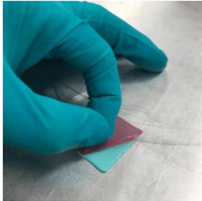
2. Place the exposed side of the gap filler on the desired substrate by applying slight force to ensure the gap filler sticks.
