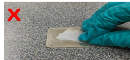
DO NOT peel the tape back on itself 不要向后撕扯胶带
