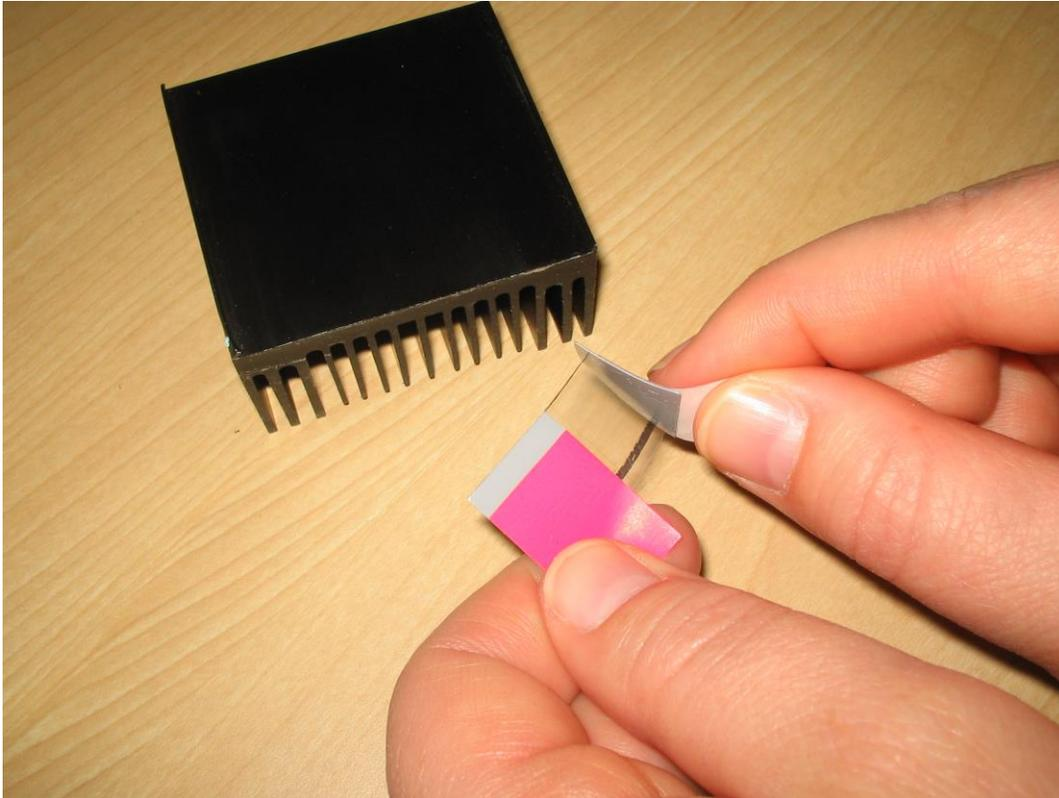
2. Carefully align and place the pad with the top tabbed liner onto a clean thermal solution mounting surface. Apply finger pressure across the entire surface of the pad to remove any trapped air between the pad and the thermal solution.
