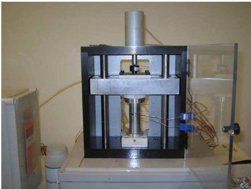
Picture #4 ASTM D5470 thermal resistance tester
