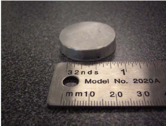
Picture #1 Aluminum disk used for reliability testing
